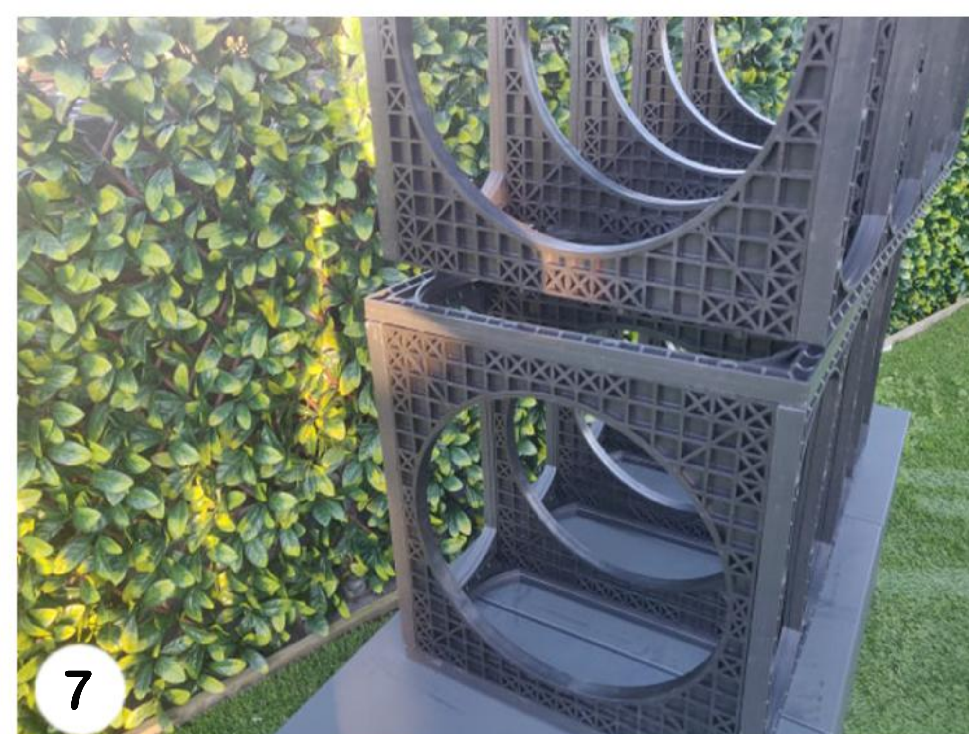
7 Repeat steps 3 & 4 above (remember to use a large Ellipse plate if you are looking to block off one side) but this time leave the top and bottom open. Lower this crate (with one of the open faces pointing downwards) onto the first crate and fix in place.
