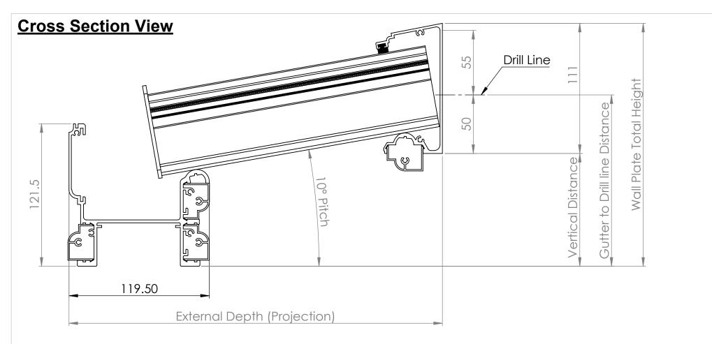
Example distance to appropriate drill hole on wall plate 10 degree roof pitch.
